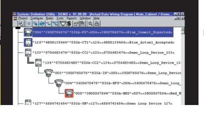
Signature Series input/output modules are powerful yet flexible devices that allow the life safety system to interact with the world beyond its Signature loop controller. The function of each module is determined by an installerselected personality code, which is set during system configuration. This exclusive Signature Series innovation provides elegant system interoperability at a fraction of the cost and time when compared with other methods.
