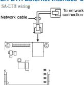
The SA-ETH card provides a standard 10/100 Base T Ethernet network connection for connecting to an intranet, a local network, or the Internet. The card can be used to download configuration programming from the iO-CU to the panel over the network.
